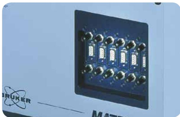
If more analysis points need to be monitored, the external 6-channel multiplexer provides a convenient way to further expand the multi-point analysis capabilities of the MATRIX-F. It features a sequential, precise optical switching mechanism, similar to the internal multiplexer, for accurate and reliable measurements. The external multiplexer is equipped with connectors for fibers with SMA and BQC type.
