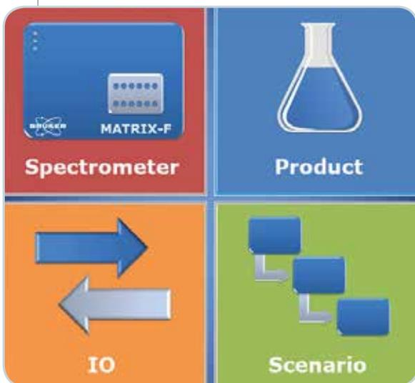
Inside the scenario setup everything is combined. It allows the user to assign a specific spectrometer, with a specific measurement channel to a specific product. If necessary external triggers can be defined which allow the user to integrate the results of CMET into a process control software.
